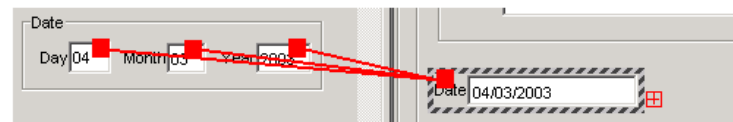
(3) After finishing the one-to-one direct copying, click on the minus sign on the right side of the Date field in the target form, the sub-form disappears. The lines between the source fields and the target field indicate the many-to-one mapping specification
