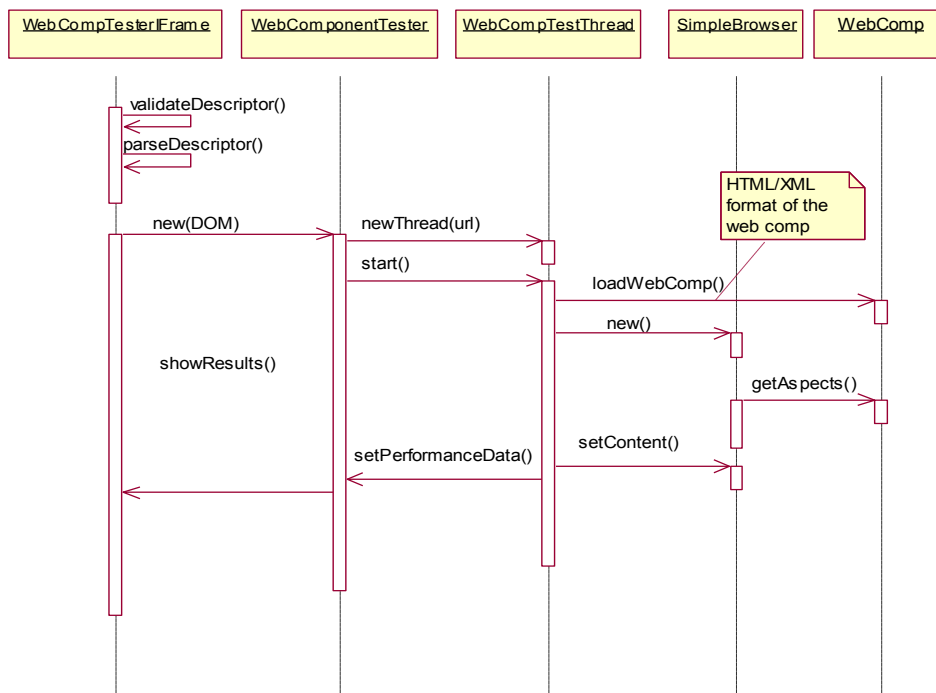
Figure 8-9 Web component aspects testing tool sequence diagram
