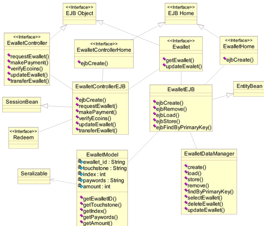
Figure 6-15 E-wallet enterprise beans (server-side) class diagram
