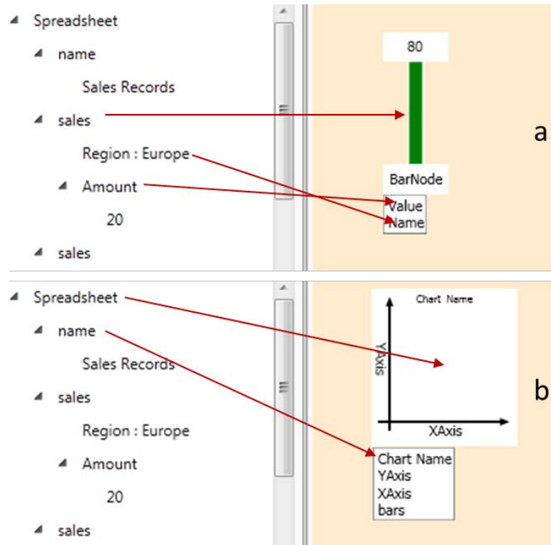
Figure 4.9 Mapping sales records input to notations: a) Mapping a sales record to a bar, b) Mapping spreadsheet to chart. Arrows depict drag and drop directions.
