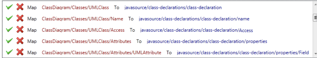
Figure 9: Sample of resulting suggested correspondences between UML class diagram and Java code visualization.
