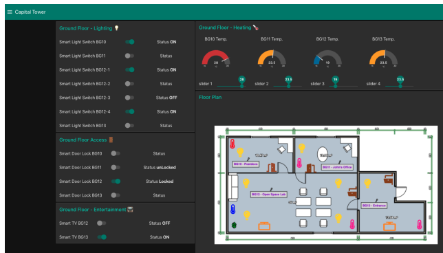
Figure 6: Node-Red Dashboard for the HumaniSe Lab (with floor map integration)
