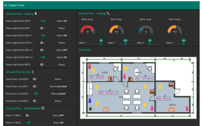
Figure 7: Node-RED Dashboard for the HumaniSe Lab (with floor map integration)
