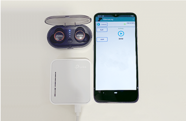
Figure 6: Each participant received a package containing the GustosonicSense system that consists of the earbuds, the smartphone with our customized application, and a router.
