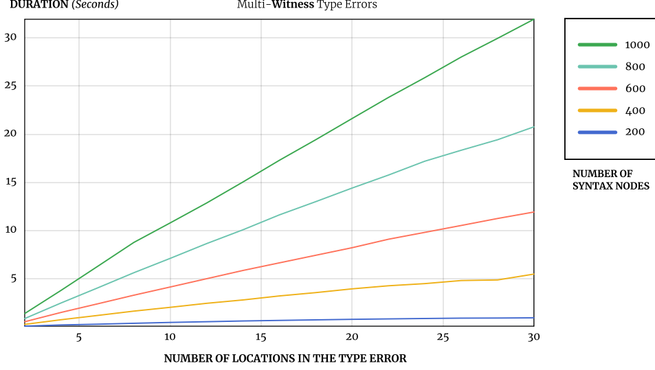
Fig. 24 Impact of Multi-witness Type Errors on Performance. Similar to evaluating multi-step type errors, we generated five sets of programs differentiated by program length: Set 1 consists of 200 nodes, Set 2 consists of 400 nodes, Set 3 consists of 600 nodes, Set 4 consists of 800 nodes, and Set 5 consists of 1000 nodes. For each set, we initiate with a multi-witness type error 1/3 witness, that is, 1 witness on one side of the type error and 3 on the other, and gradually increase up to 1/30 witnesses. This figure illustrates the time required to generate type error diagnostics with respect to the number of witnesses involved in a type error.
