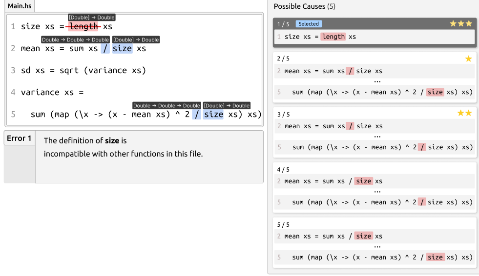
Fig. 9 Goanna's Error Grouping. This error, although its potential offending parts appear in many declarations, is possible to fix in one place, i.e., by changing the definition of the size function on line 1. Therefore, Goanna reports it as a single error.
