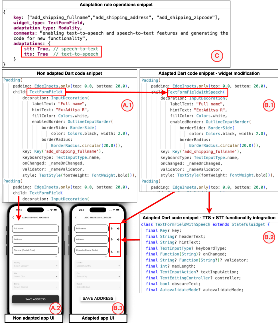
Fig. 10 An example of multi-modality adaptation with source code transformation. The previous presentation adaptation example is extended to integrate text-to-speech and speech-to-text functionality for the defined TextFormField widgets. In (C), when the speech-to-text and/or text-to-speech properties are set to true, the MDE pipeline identifies the relevant widget (A.1) and adapts the source code to include the necessary functionality, as shown in (B.1) and (B.2). This transformation is reflected in the app's front end, where the adaptation evolves from instance (A.2) to (B.3).
