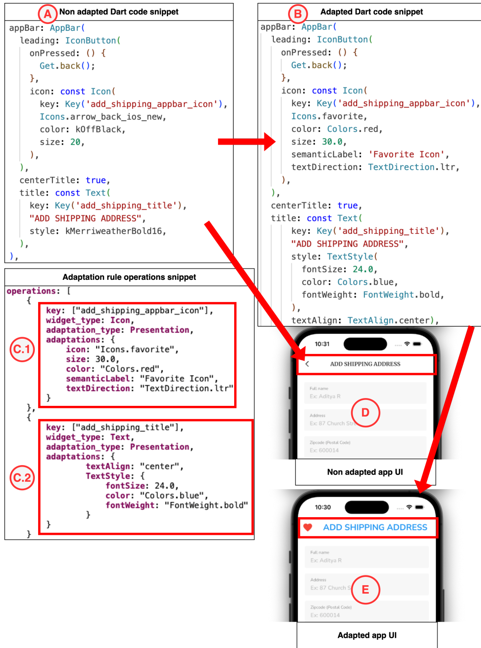
Fig. 8 A simple source code transformation example of a presentation adaptation . In this example, two Flutter widgets (Text and Icon) within an AppBar are transformed. The original app (D) and its source code (A) were sourced from an open-source GitHub repository. The MDE pipeline applies the specified adaptation rules operations (C.1 and C.2) to modify the property values of each Flutter widget (B). The adapted app instance (E) now reflects the changes defined in (C.1) – Icon widget and (C.2) – Text widget.
