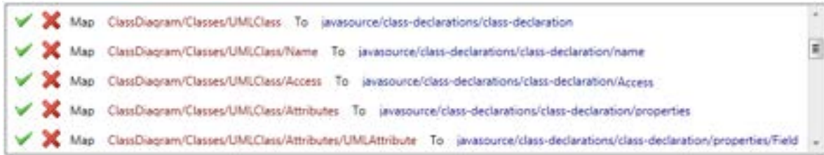
Figure 9: Sample of resulting suggested correspondences between UML class diagram and Java code visualization.
