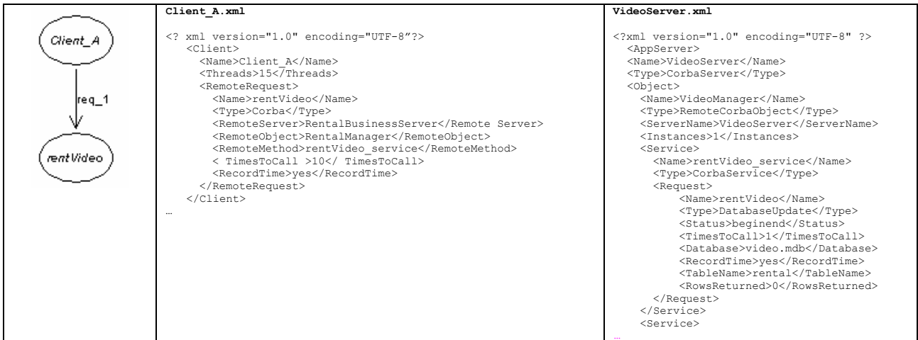
Figure 12. (a) Part of architecture model; (b) XML encoding of some of model.
